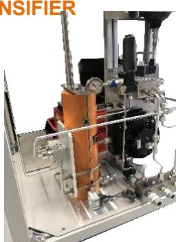
The confining pressure intensifier is a high-precision, servo-controlled pressure system designed to apply and maintain stable confining pressure during triaxial testing.
