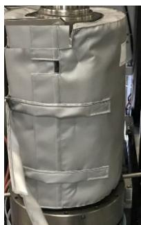
The heating jacket is a precision-controlled thermal system designed to uniformly heat rock specimens during triaxial testing.
