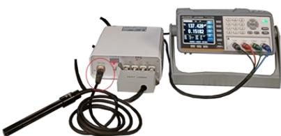
The electrical resistivity system is an integrated measurement module designed to evaluate the electrical properties of rock specimens under triaxial stress conditions.
