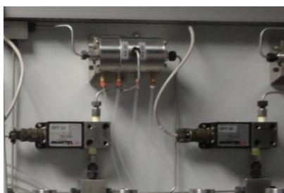
The permeability system is a high-precision module designed to measure fluid flow through rock specimens under controlled stress and pressure conditions.
