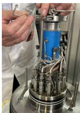
The acoustic emission system is a high-sensitivity monitoring module designed to detect and locate microcracking and fracture events during triaxial testing.
