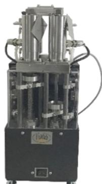
The pore pressure pump is a high-precision, servo-controlled unit designed to apply and regulate pore pressure with high accuracy during triaxial testing.
