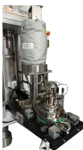
The triaxial cell is a high-pressure vessel designed to provide precise confinement and axial loading for triaxial and unconfined compression tests.
