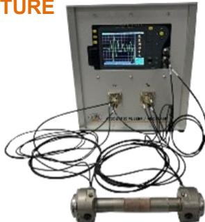
The ultrasonic velocity system is an integrated measurement module designed to determine P- and S-wave velocities in rock specimens during triaxial testing.
