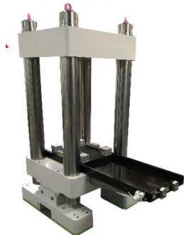
The hydraulic compression frame, built with four high-stiffness columns, ensures maximum rigidity and alignment accuracy while applying precise axial loads to specimens mounted in a triaxial cell. A servo-controlled hydraulic actuator, integrated in the upper crosshead provides great loading capacity. The frame can be operated under both static and dynamic testing conditions.
